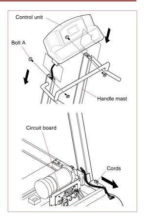
Attach the connectors on the 3 cord ends to the circuit board inside the main body.
